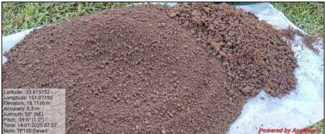
Photograph 9: Fill soil matrix observed in TP105, after 10L asbestos quantification. Dated 14/01/2025.
