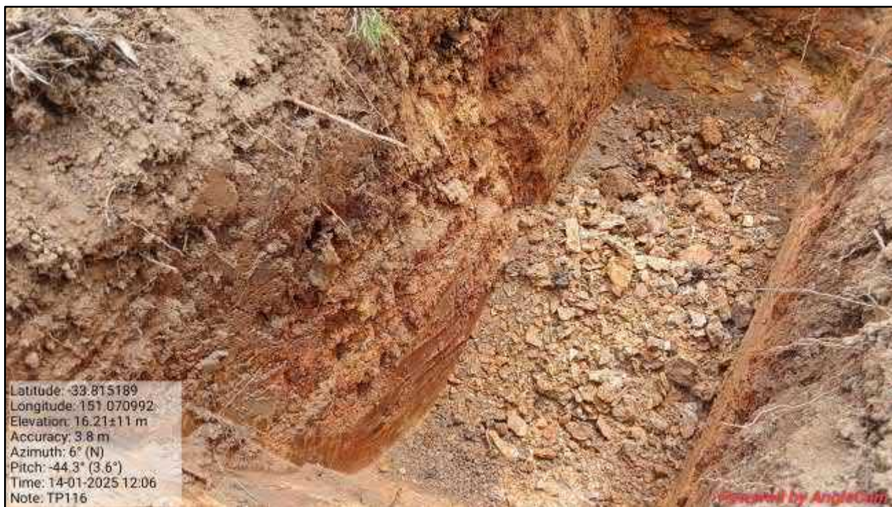
Photograph 7: Soil profile encountered within TP116. Dated 14/01/2025.
